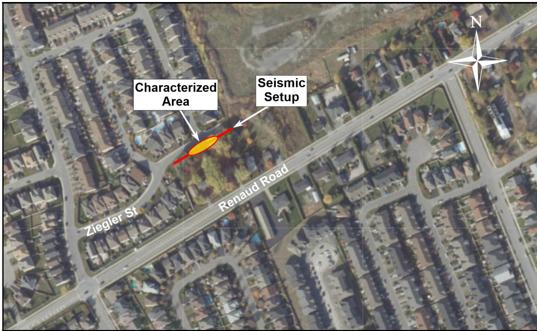
Figure 2: Location of the Seismic Lines (source: GeoOttawa )
