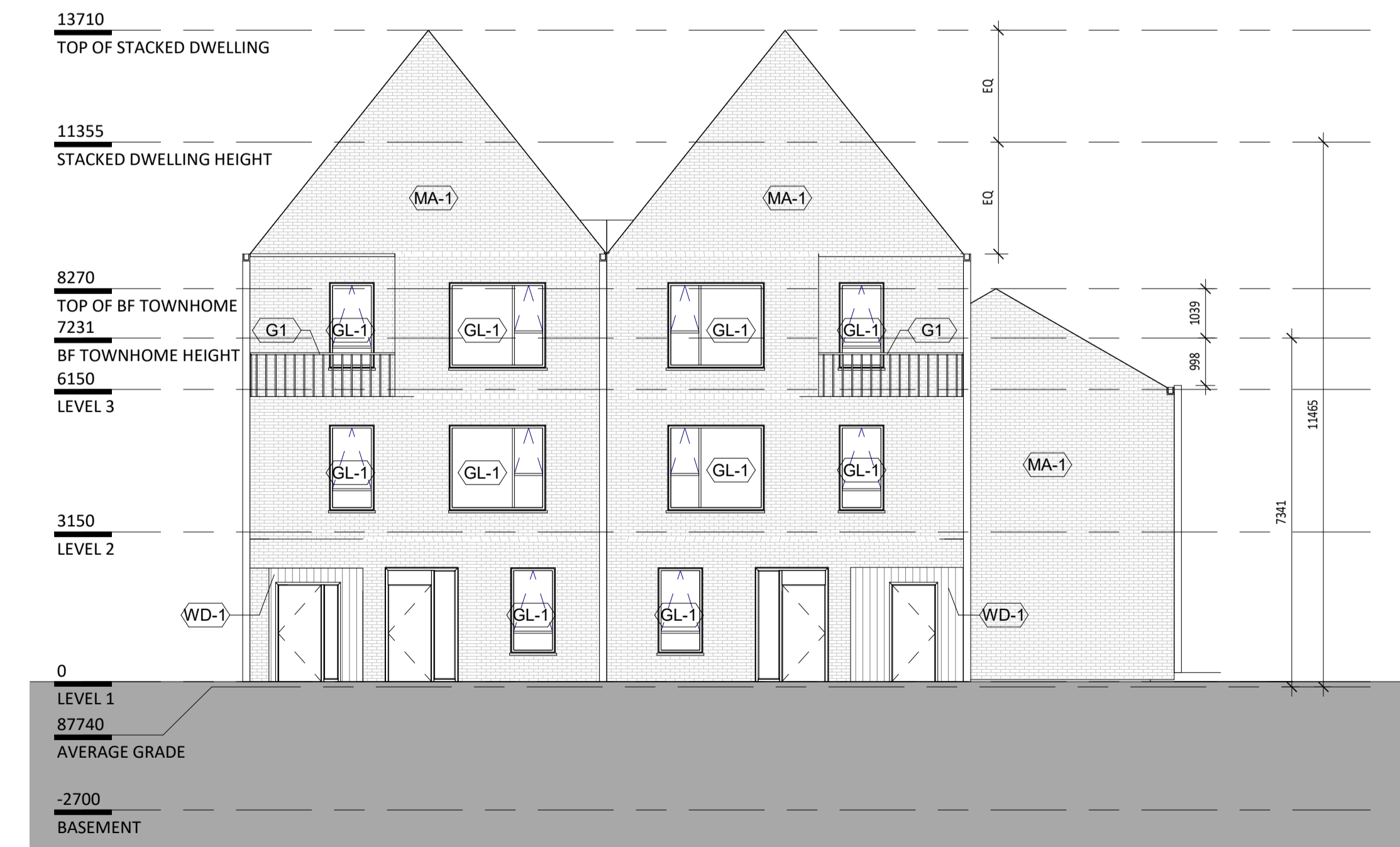
4 BLOCK 1 - WEST ELEVATION 1:100
