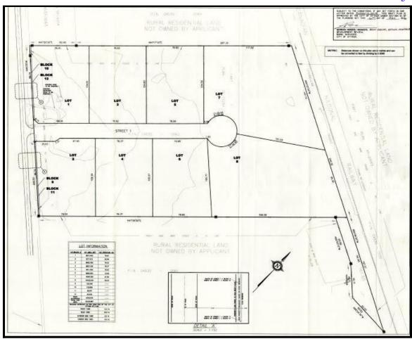
Draft Plan of Subdivision with 8 rural residential lots all at least 0.8 ha in size and with a drainage outlet at the south east corner of the overall property. Dunrobin Road on the left hand side of the image (west side) and former rail corridor on the right hand side
