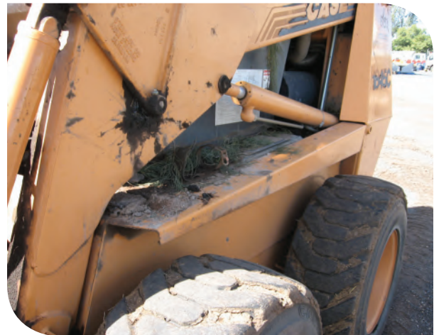
Plant material attached to bobcat.
