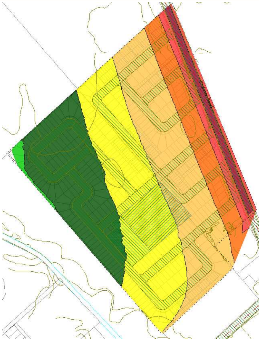
FIGURE 5: NIGHTTIME TRAFFIC NOISE CONTOURS (1.5 M ABOVE GRADE)
