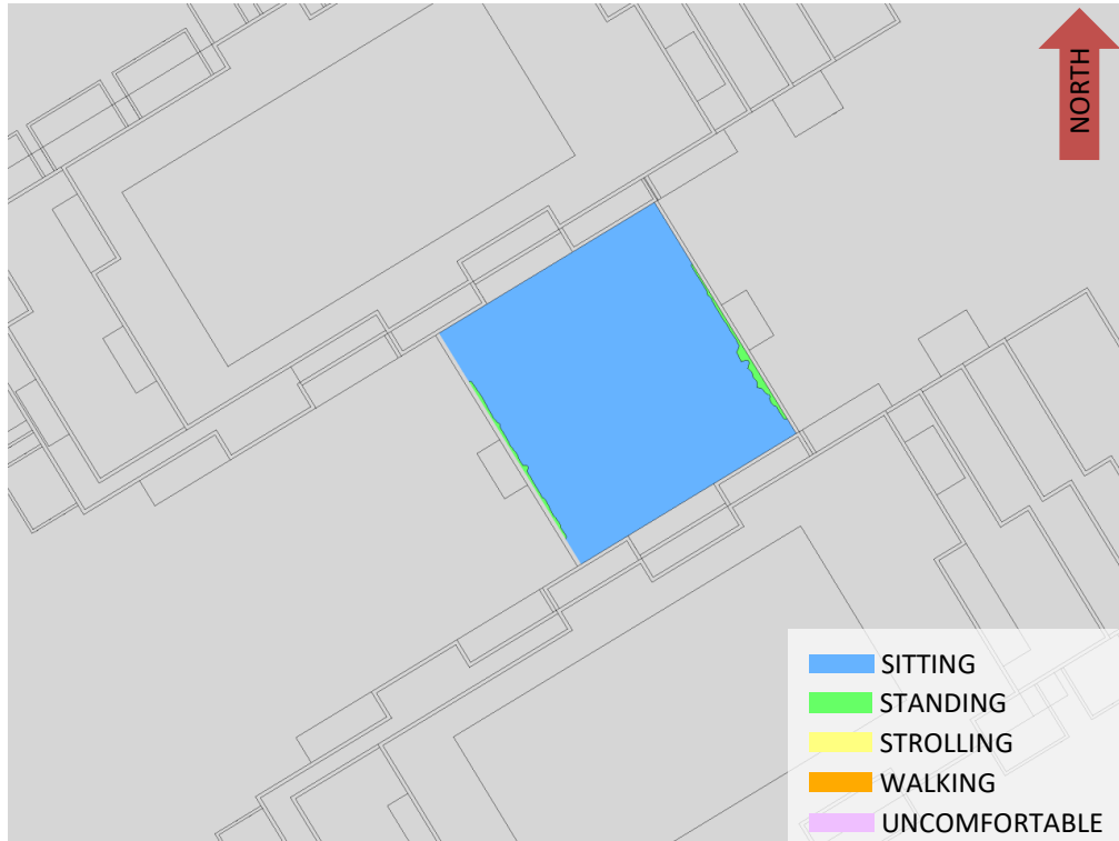
FIGURE 5A: SPRING – WIND COMFORT, LEVEL 2 AMENITY TERRACE
