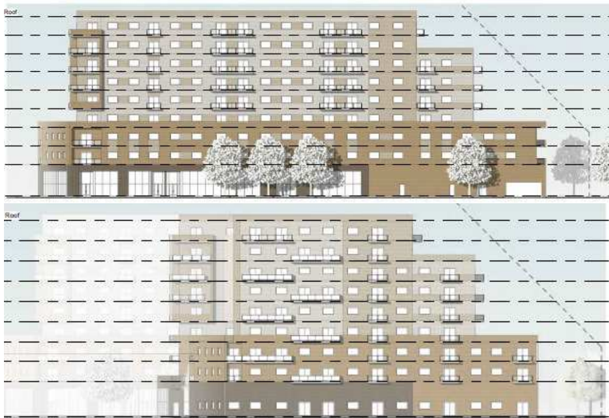
Figure 11. West elevation of Building A (top) and Building C (bottom), showing the 45-degree angular plane applied from the rear property line
