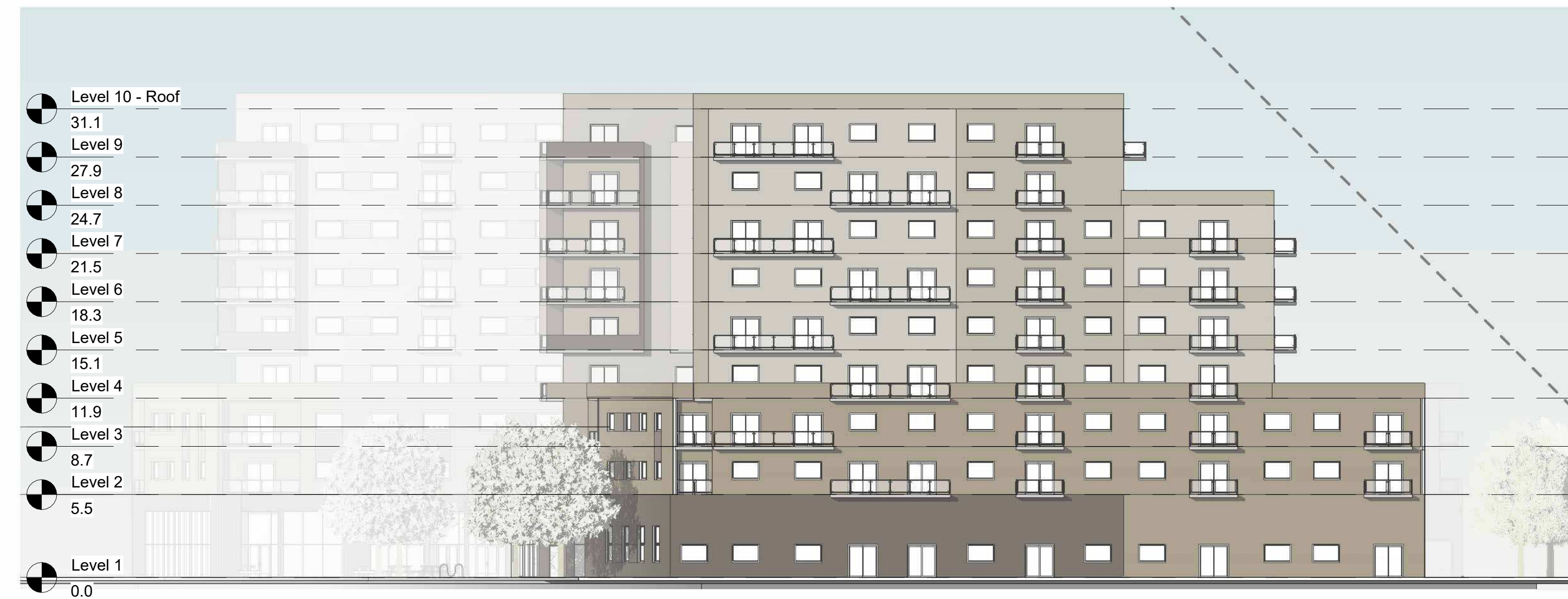
BUILDING A - WEST ELEVATION 1 : 250
