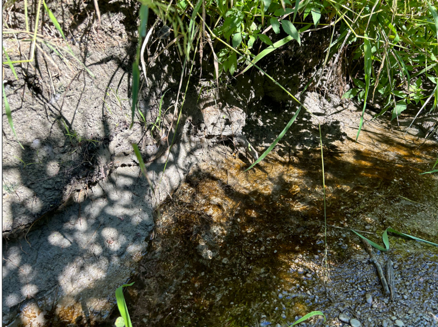
Photograph taken facing the right bank. Bank materials were composed of thick and loose clay deposits. Undercutting of up to 15 cm was observed along the right bank.
