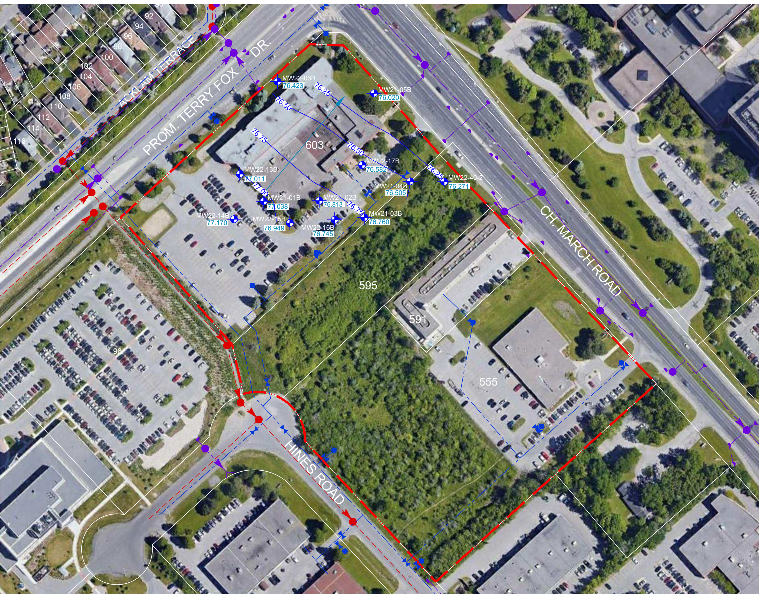
FIGURE 3B GROUNDWATER ELEVATIONS AND INTERPRETED FLOW BETWEEN 9.1 AND 13.7 mbgs
