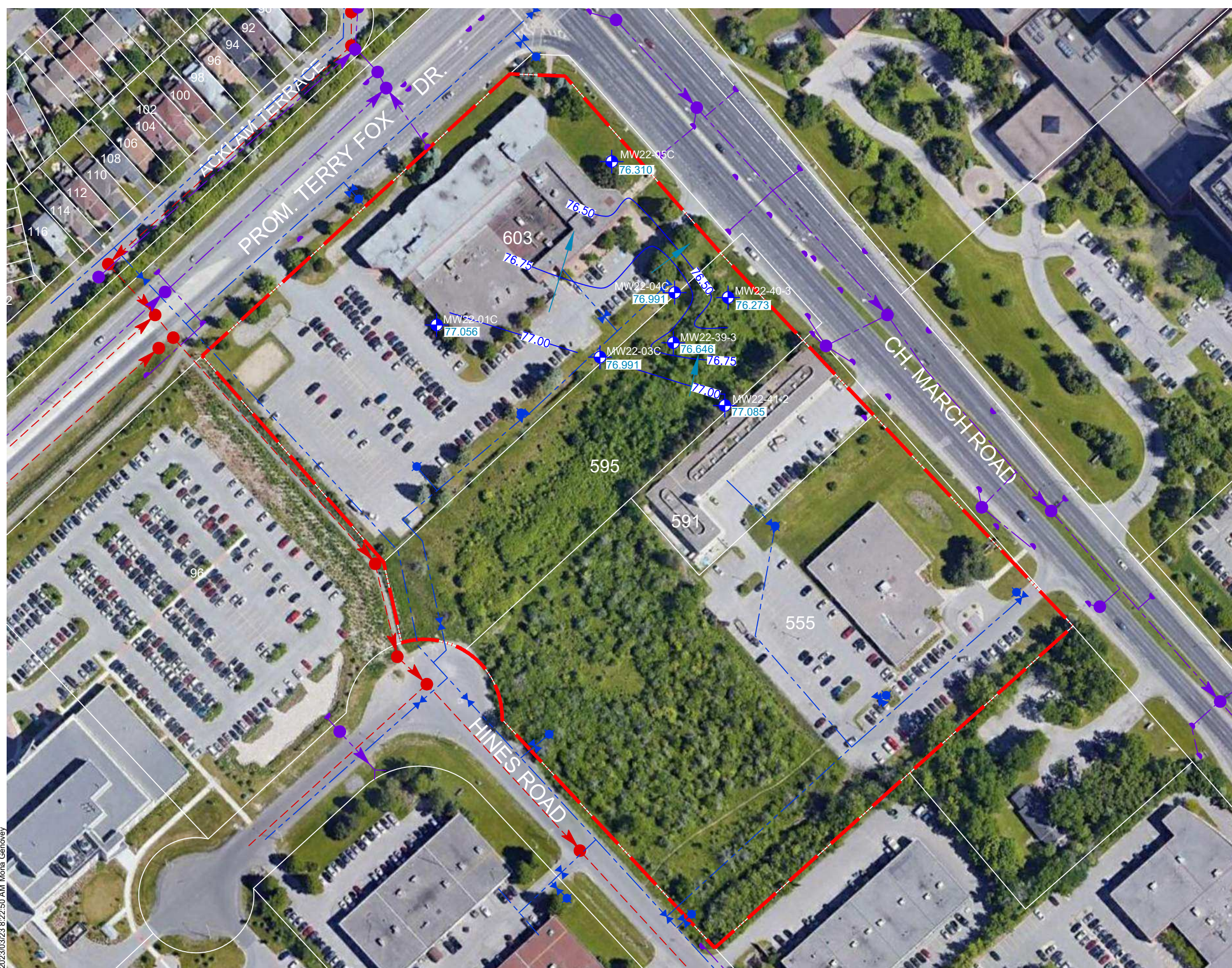
FIGURE 3C GROUNDWATER ELEVATIONS AND INTERPRETED FLOW BETWEEN 13.7 AND 18.4 mbgs
