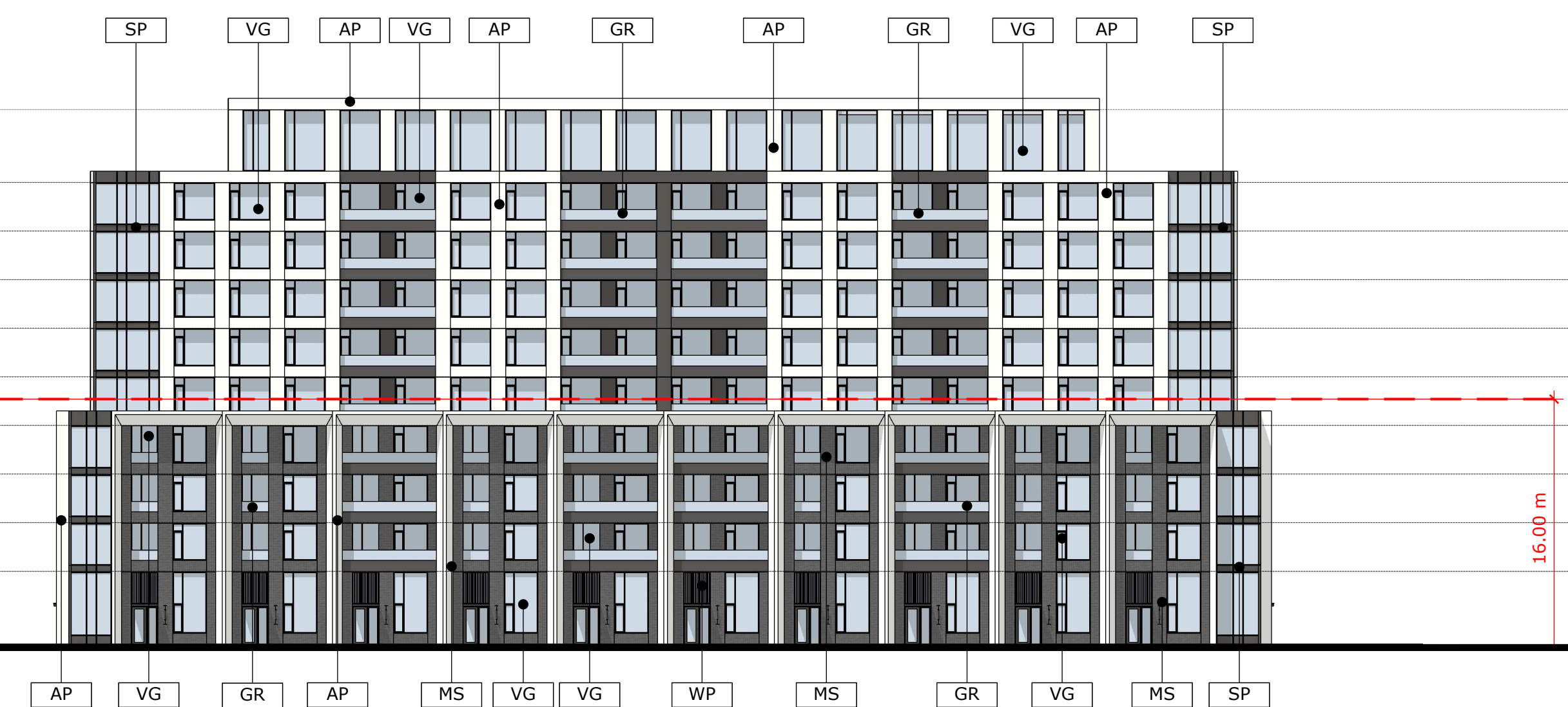
4 BUILDING 3 - NORTH ELEVATION
