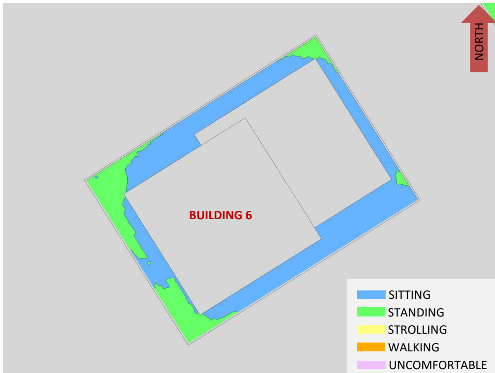
FIGURE 16B: SUMMER – WIND COMFORT, BUILDING 6 LEVEL 7 AMENITY TERRACE
