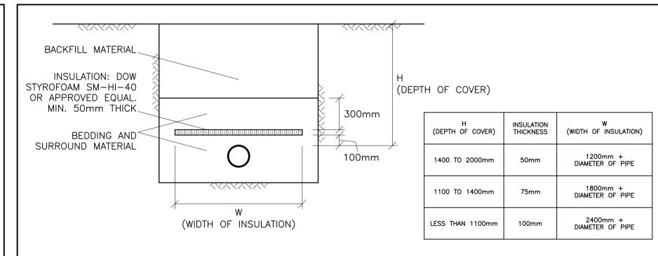
INSULATE SEWER AS INDICATED AND WHERE DEPTH
