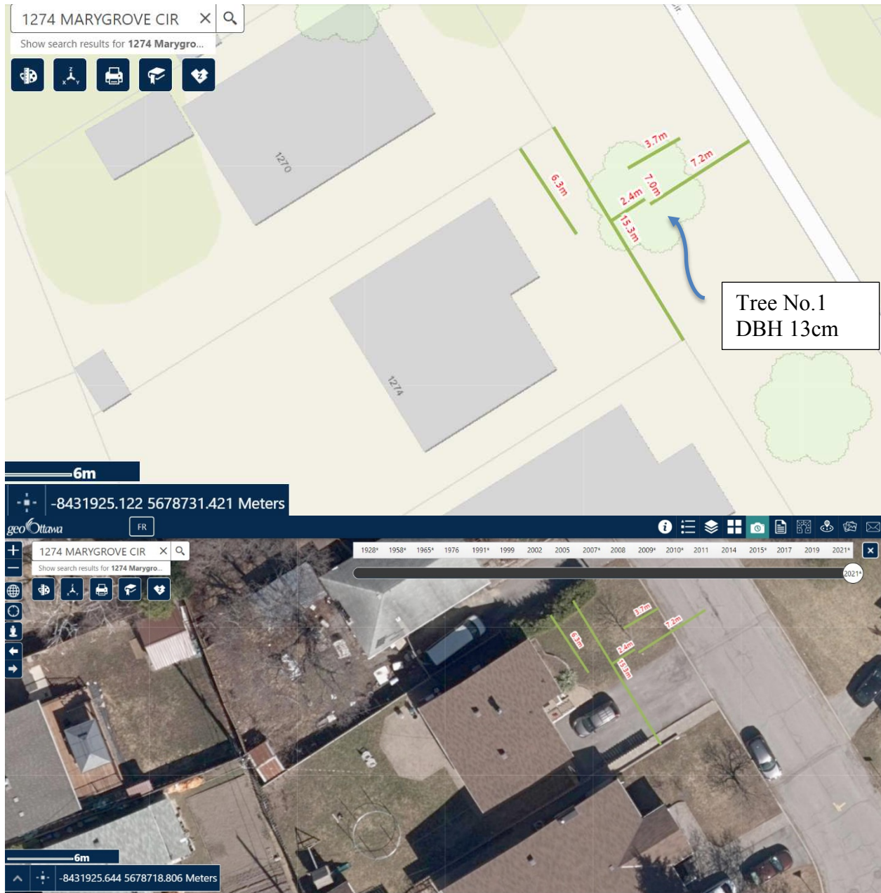
Figure 1a. Shows Parcel Base Map and Satellite Base Map respectively with existing dwelling for 1274 Marygrove Cir. Tree No.1 is 2.4 m outside the property line and 3.7m to the edge of the asphalt. (Source geoOttawa 2021)
