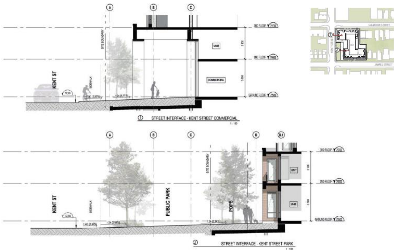
Figure 21: Sections illustrating the relationship of the building and its transition to the street at the commercial section with the projecting colonnade on the north and at the residential section of the Kent Street frontage a park in the foreground buffers the units. Source: Neuf Architecture 2023.
