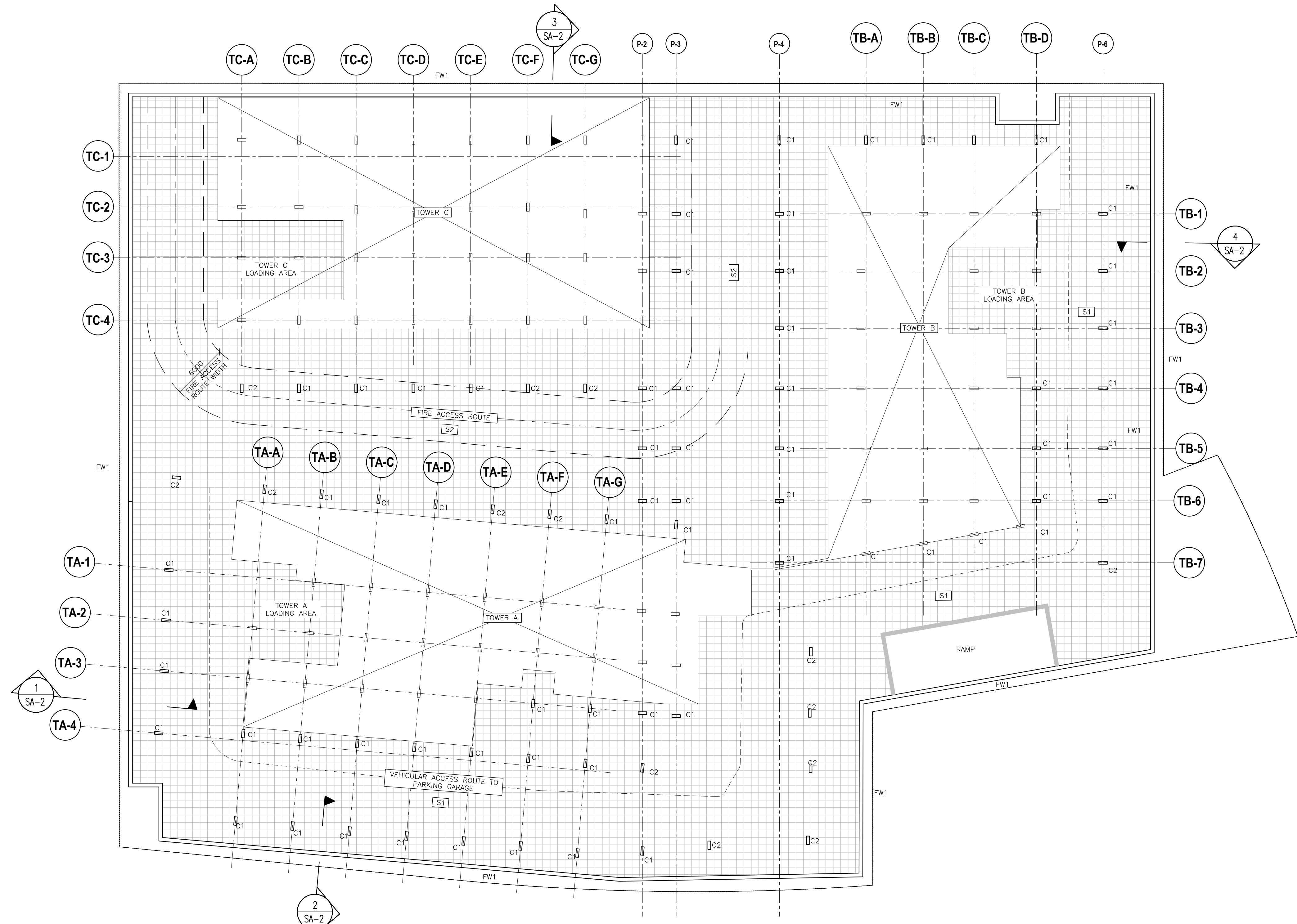
1 PARKING GARAGE P1 ROOF PLAN SA-1 1:250
