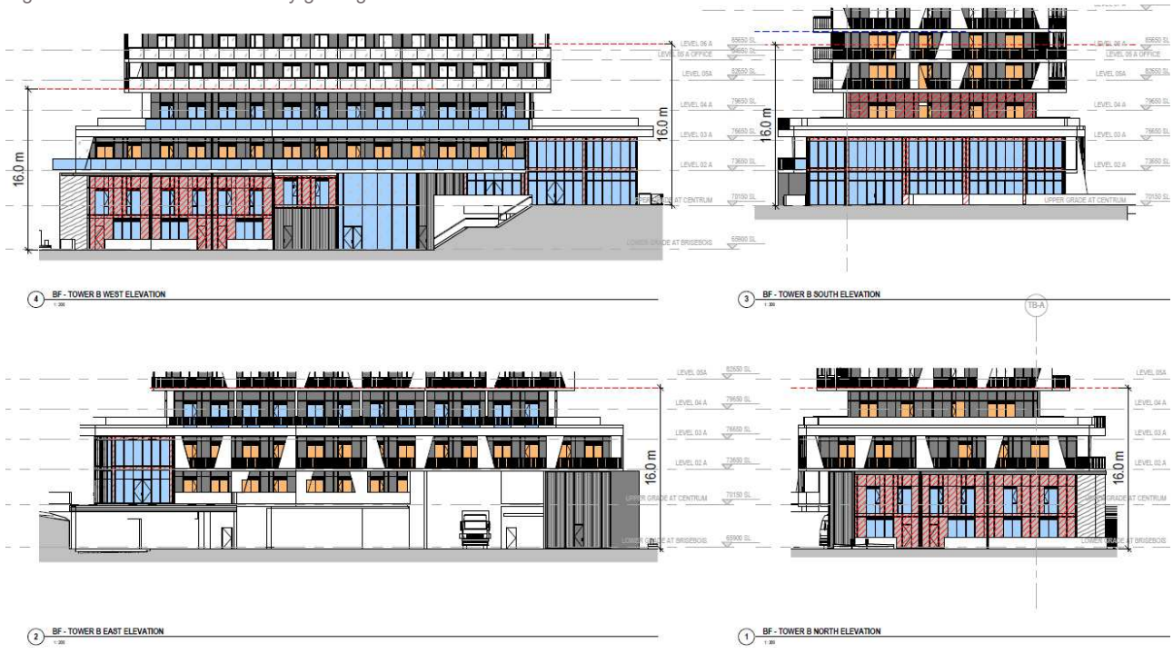
Figure 42. Tower B - Bird friendly glazing and treatment
