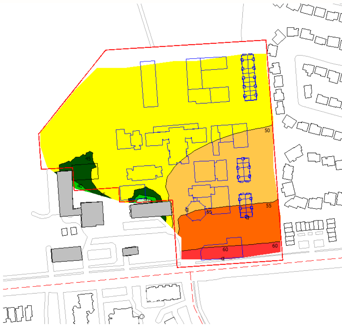
FIGURE 5: NIGHTTIME NOISE CONTOURS (1.5 M ABOVE GRADE)
