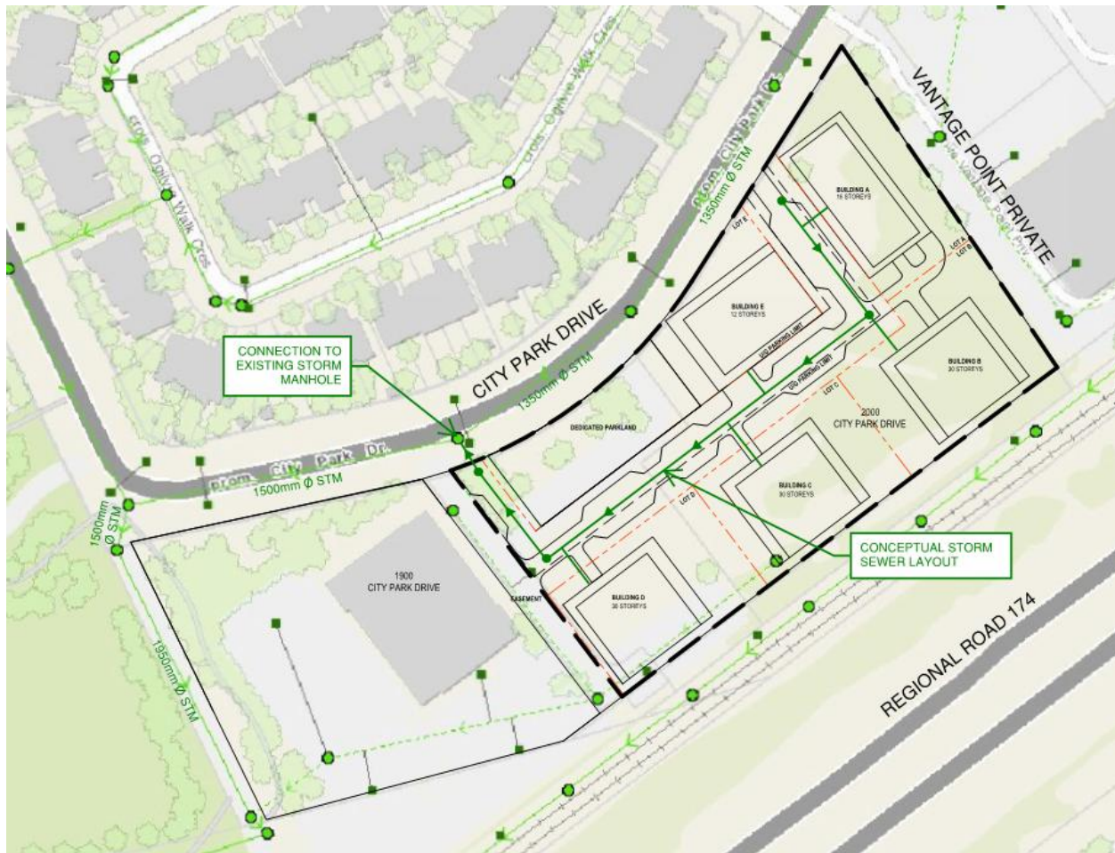
Figure 4: Conceptual Storm Servicing Layout
