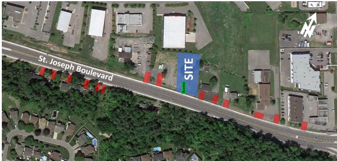
Figure 3: Adjacent Driveways within 200m of Site Access
