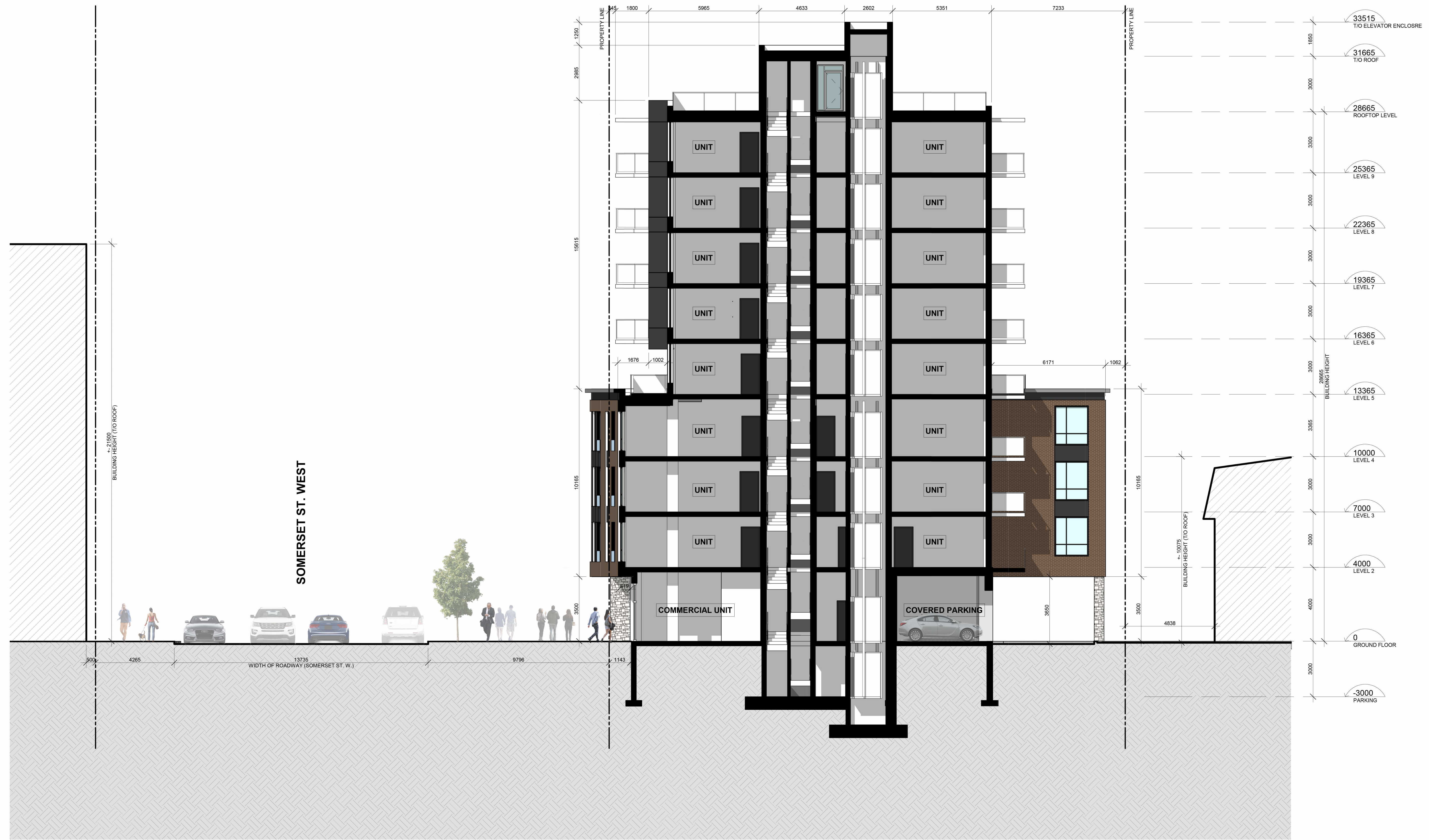
1 BUILDING SECTION 1 - SOMERSET ST. W. 1:100
