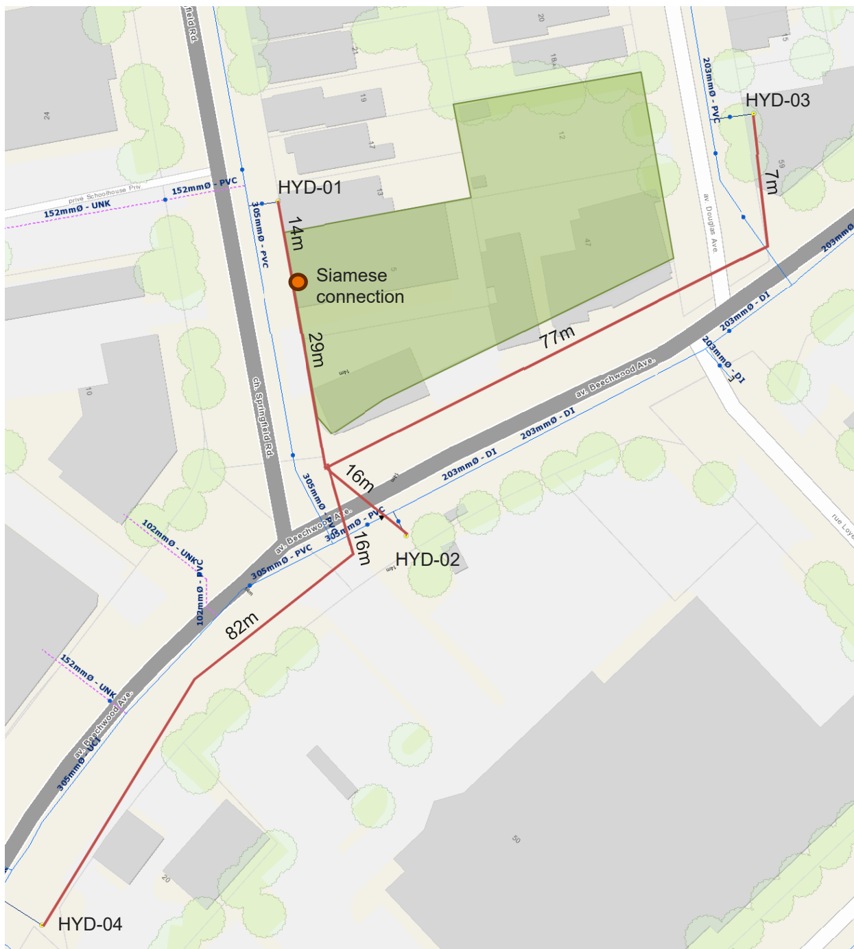
Figure 3-1: Fire Hydrant Coverage Sketch
