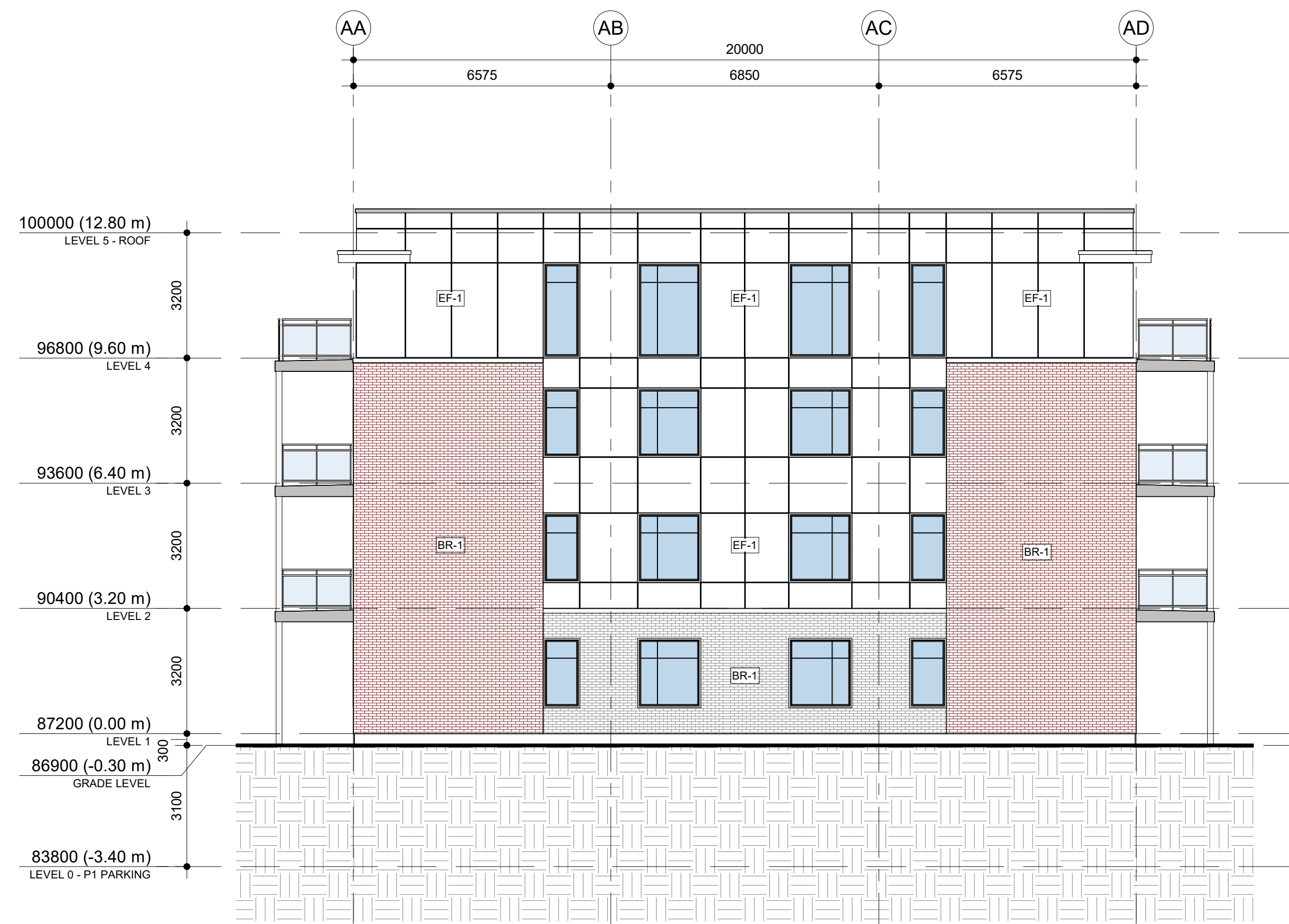
2 BUILDING A - SOUTH ELEVATION A201 1 : 100
