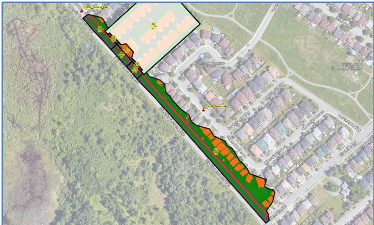
Figure 1 – Subcatchments Used for Sizing Entrance Culverts
