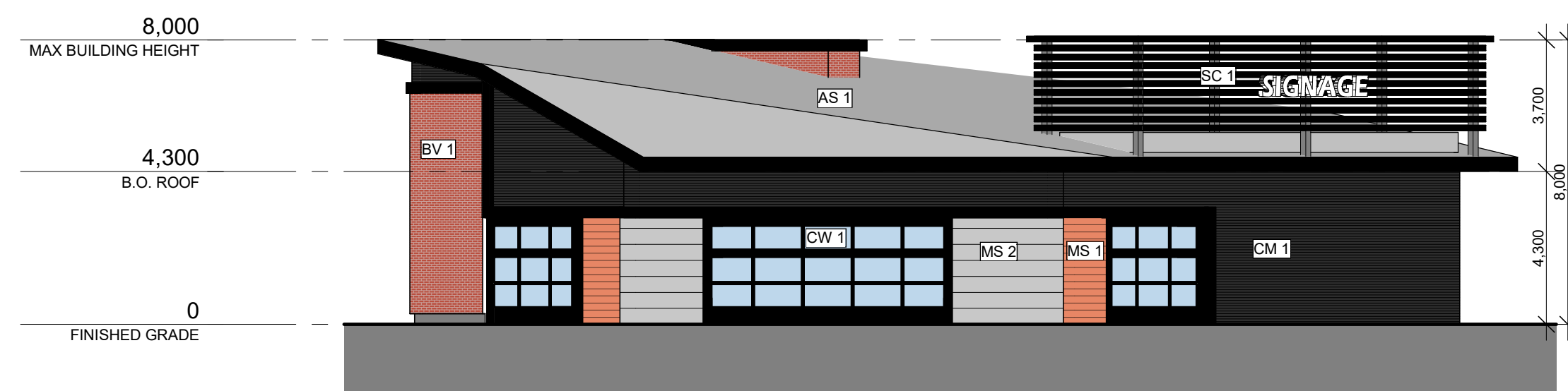
4 BUILDING C - NORTH EAST ELEVATION 1:150
