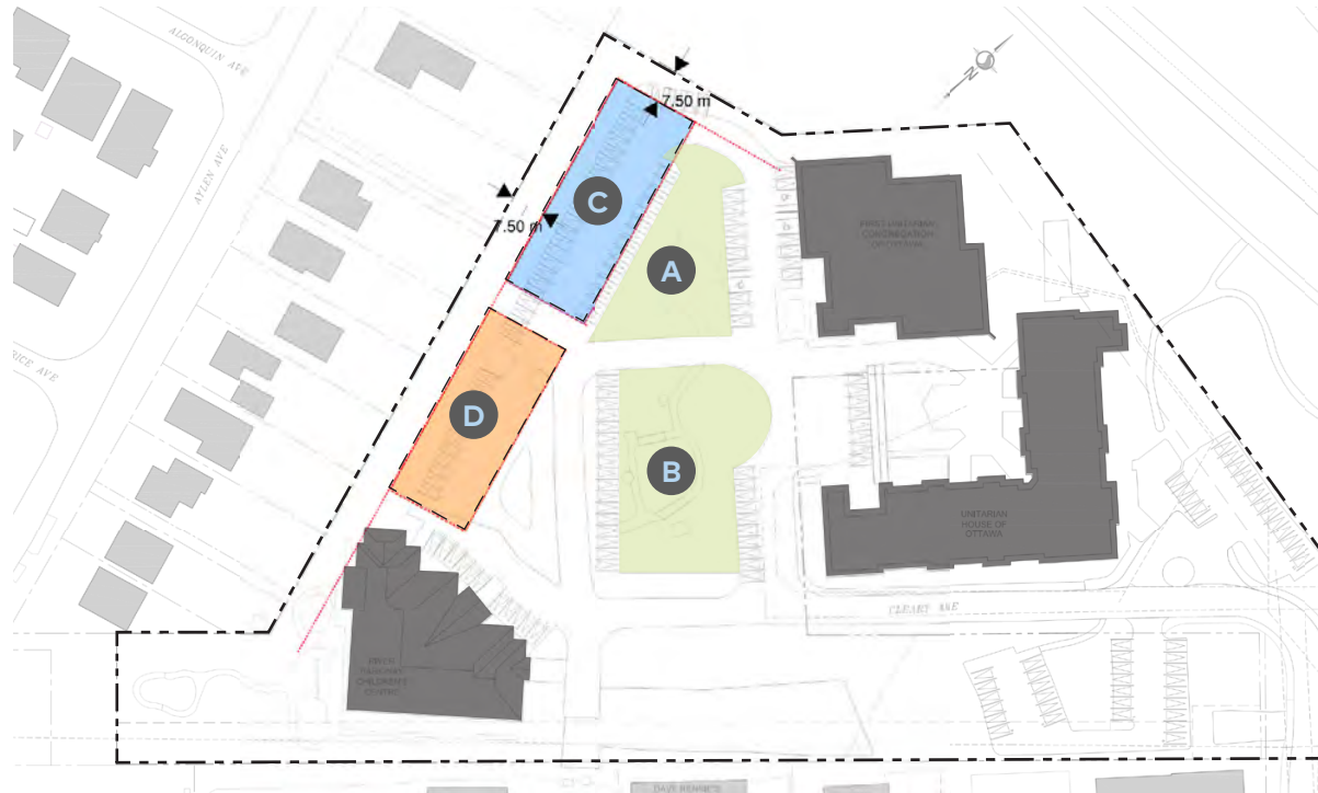
Step 1: Preliminary building placement
