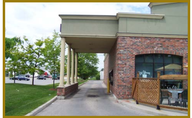
Drive-through aisles should avoid disruption to internal traffic flow, site access and pedestrian routes.
