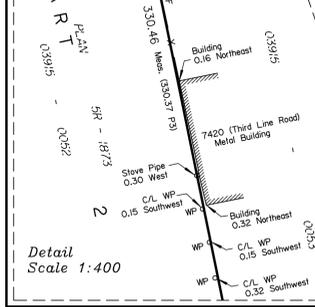
Distances shown on this plan are ground distances and can be converted to grid distances by multiplying by the combined scale factor of 0.999941.
