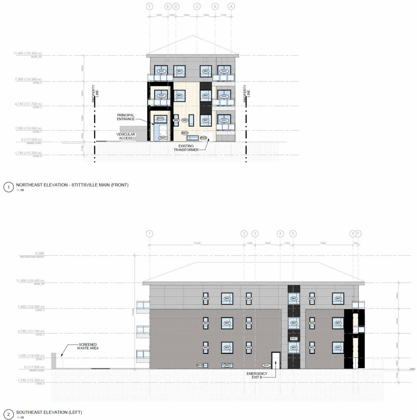
Figure 14: Elevations of Northeast and Southeast Exterior
