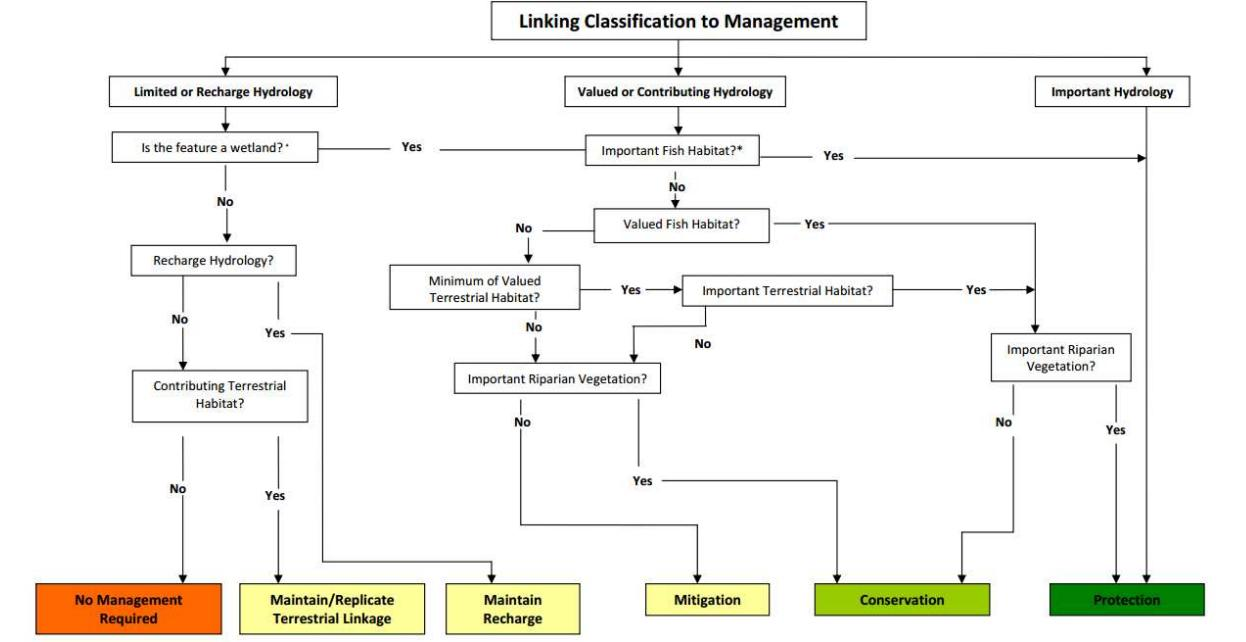
**Figure 2 Headwater Drainage Feature Assessment (HDFA) flow chart providing direction on management options**
