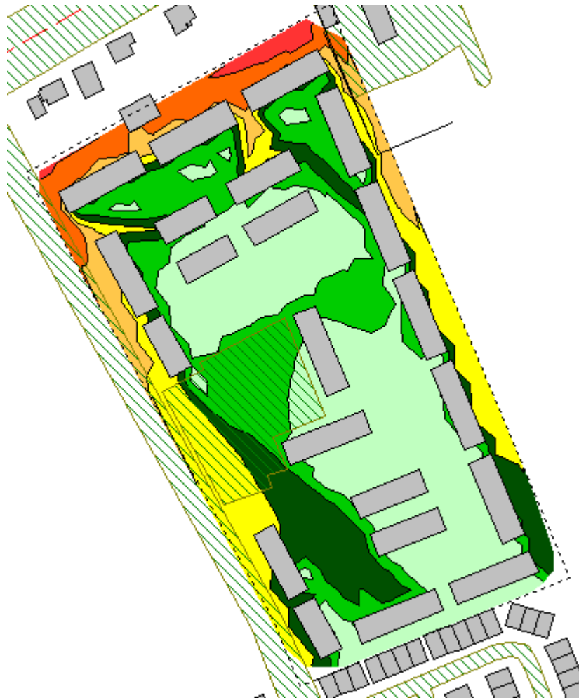
FIGURE 6: DAYTIME TRAFFIC NOISE CONTOURS (1.5 M ABOVE GRADE)
