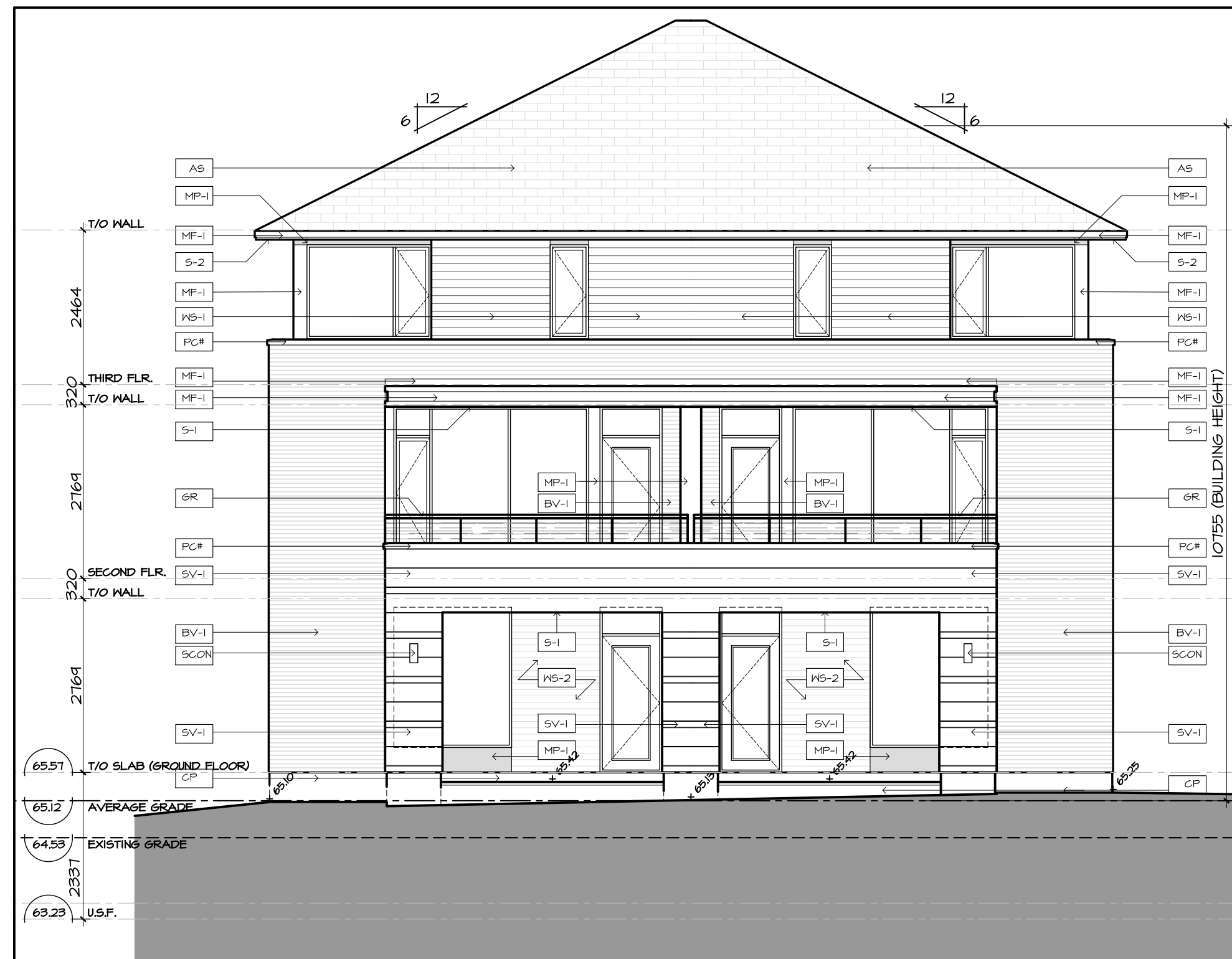
1 BLOCK T8 – NORTH-EAST ELEVATION A2.08 SCALE 1:75
