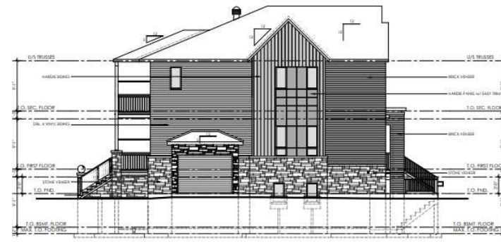
TYPICAL BLOCK - STREET SIDE ELEVATION
