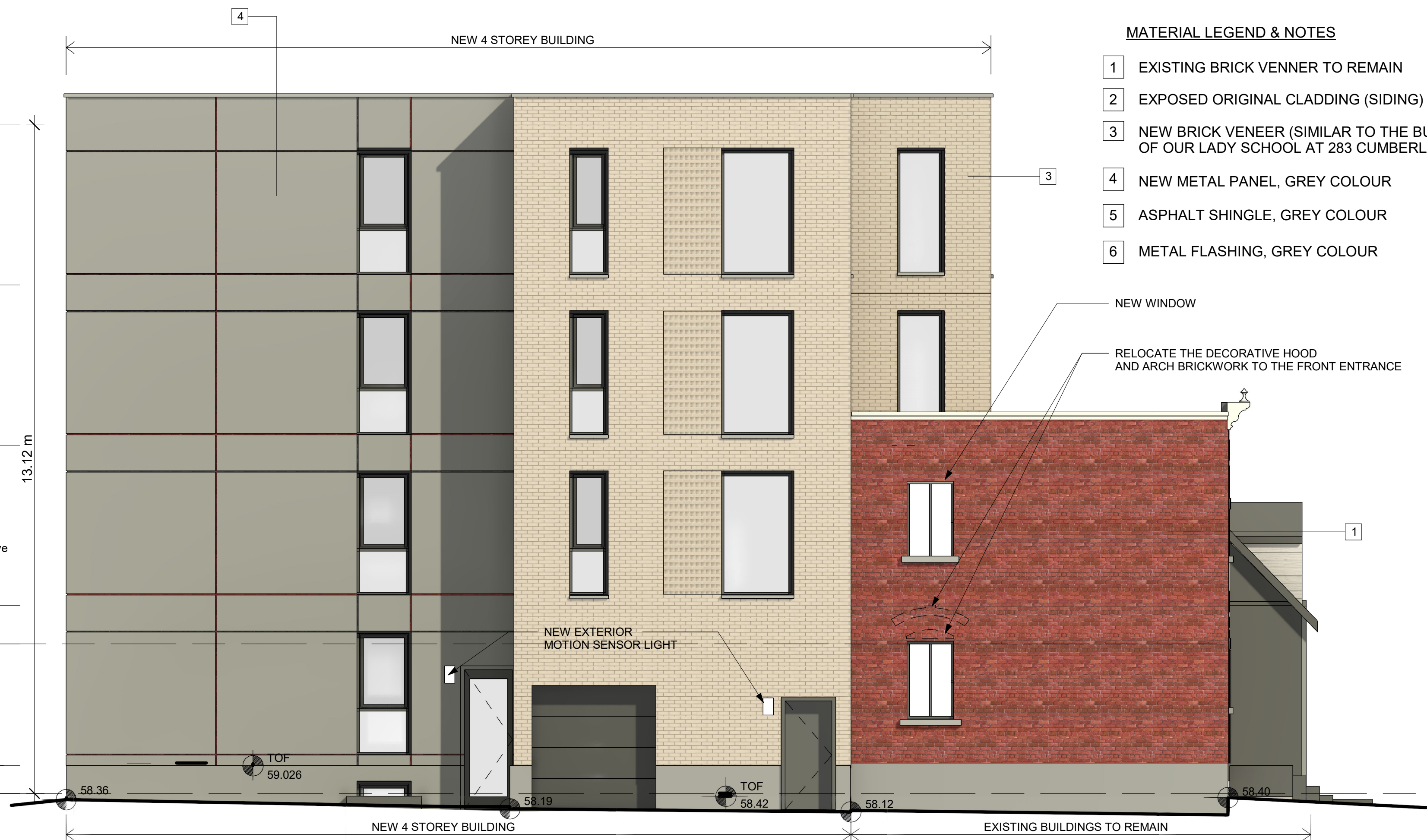
4 Side (East) Elevation 3/16" = 1'-0"
