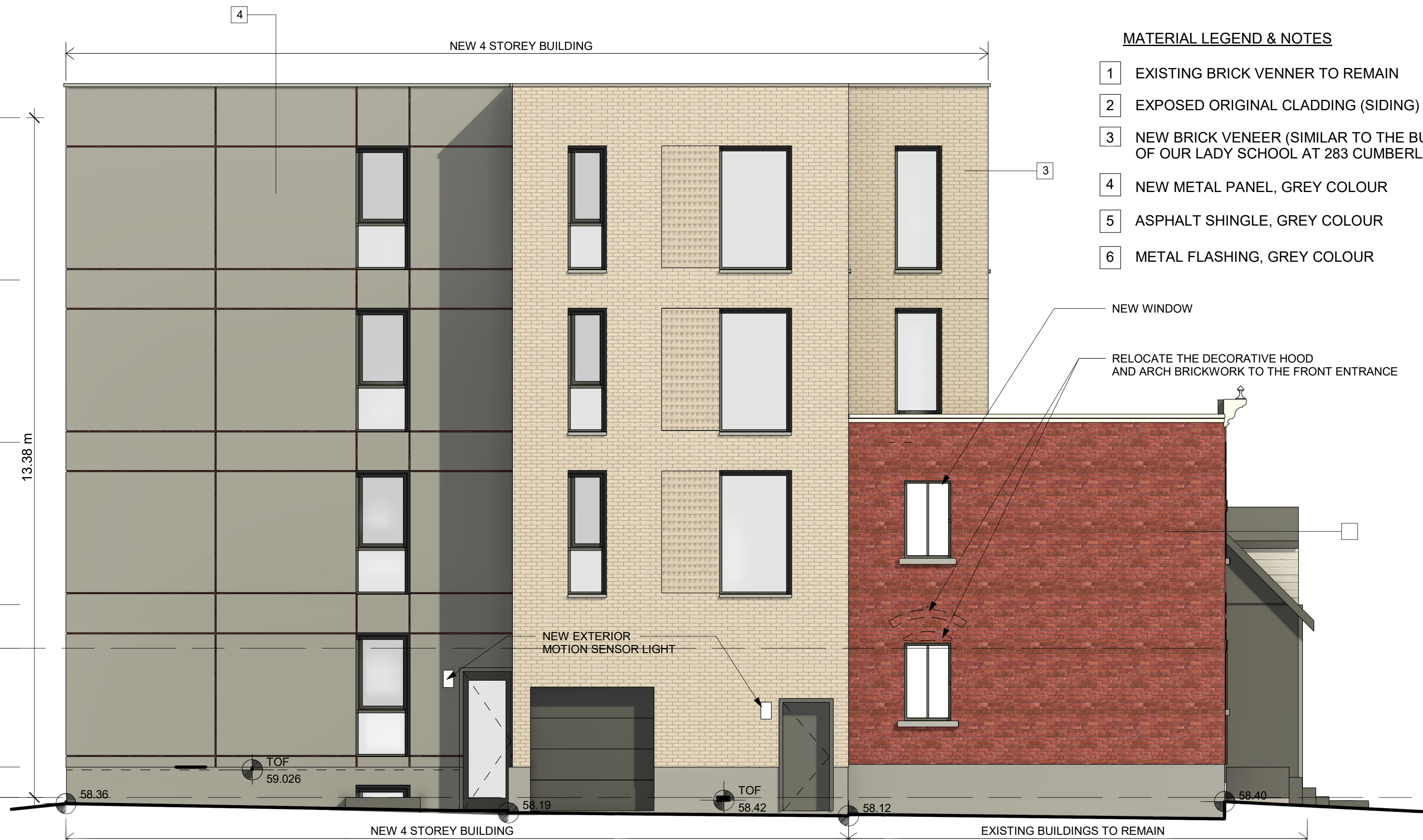
4 Side (East) Elevation 3/16" = 1'-0"
