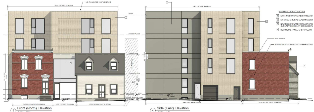
Figure 1: Elevations of the two heritage buildings being retained, with the planned 4-storey apartment setback and entered between the buildings. The two buildings have been recorded by Redline Architecture Inc.
