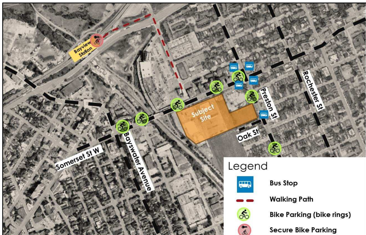
Figure 13: Design for Sustainable Modes - Existing infrastructure
