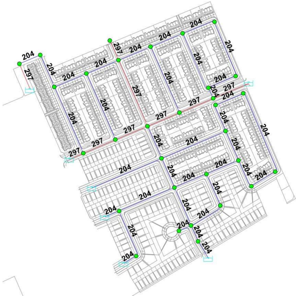
Figure 2: Watermain Layout and Connections to Existing Infrastructure
