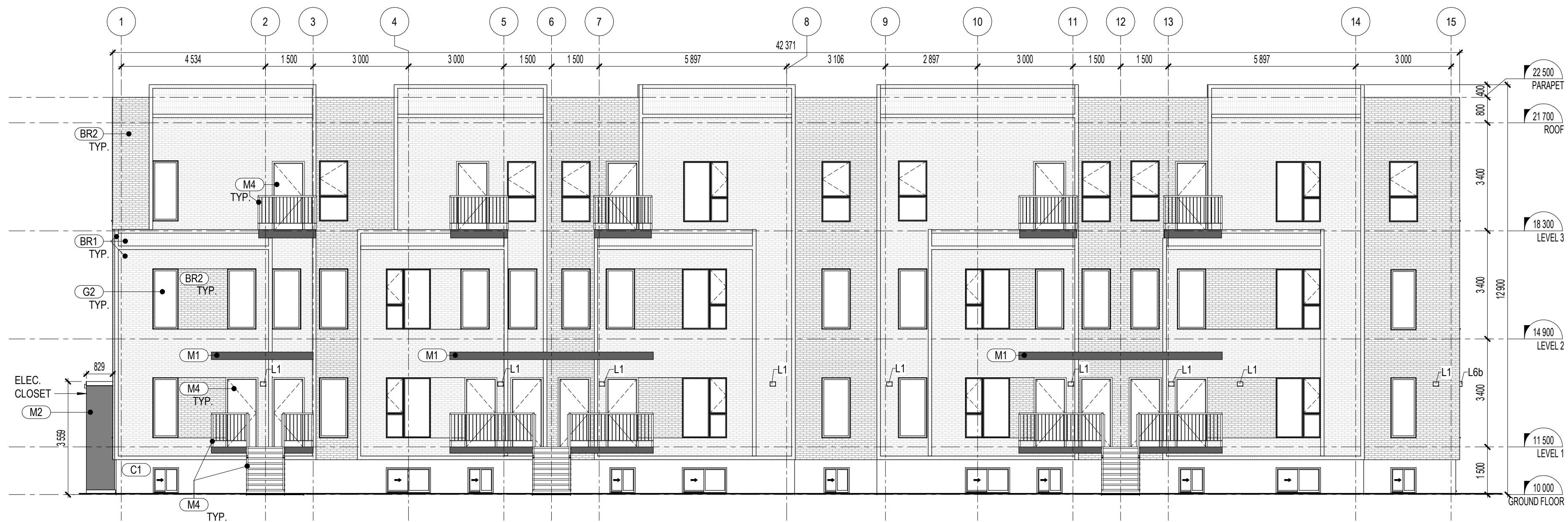
1 EXTERIOR ELEVATION TOWNHOUSE SOUTH ELEVATION A101-TH SCALE: 1 : 100
