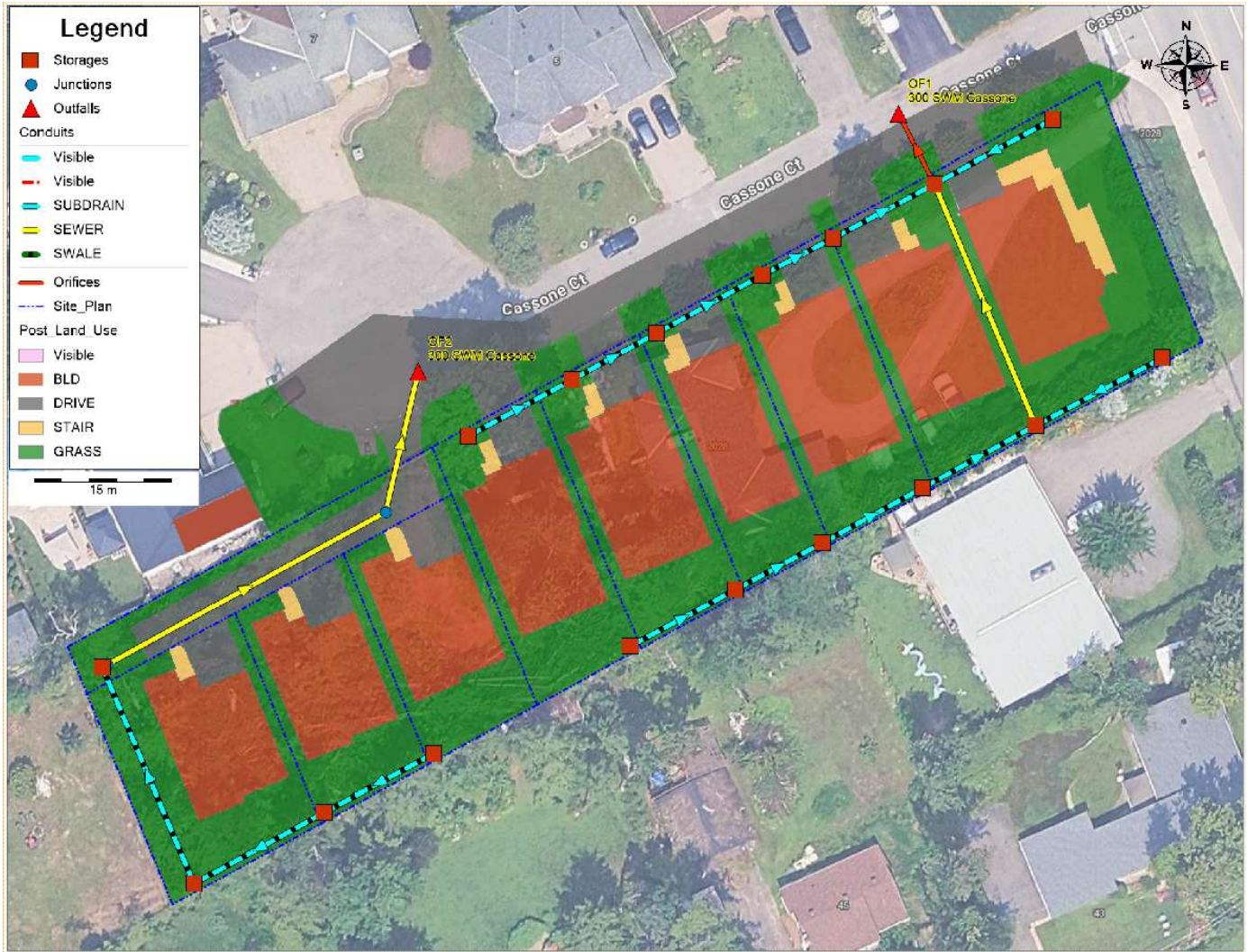
Figure 6-4: Model Schematic Showing Minor and Major System Components
