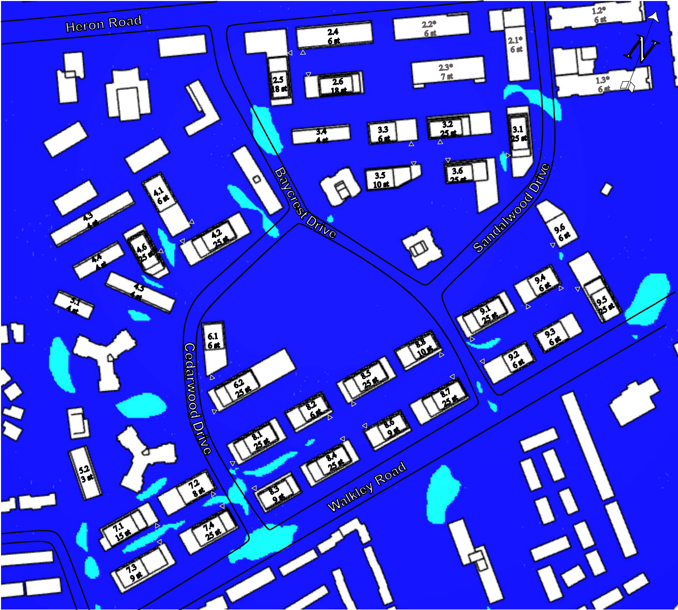
Figure 5f: Pedestrian Level Wind Velocity Comfort Categories
