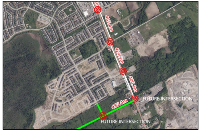
Figure 8 - Arterial Road Intersection Spacing
