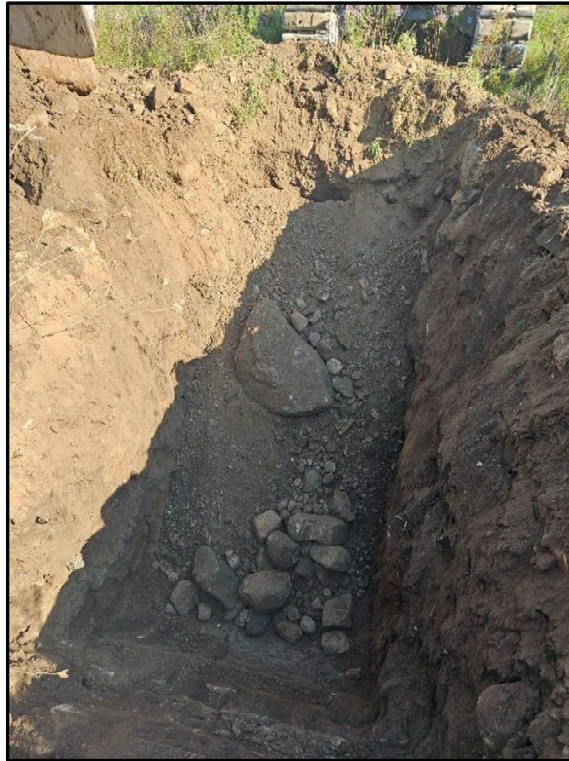
Photo 6: Photo illustrating the boulders excavated from the test pit TP 3-24.
