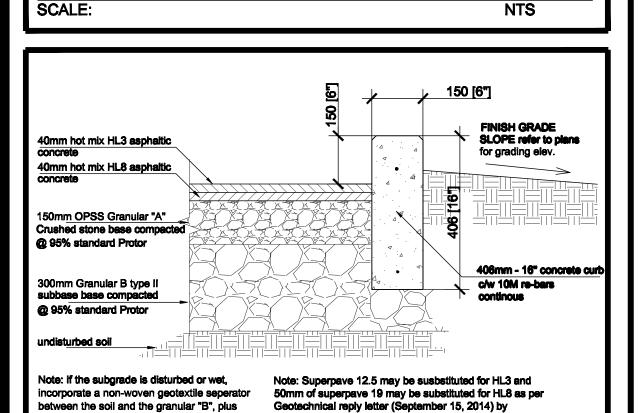
PAVEMENT STRUCTURE - HEAVY SCALE:
