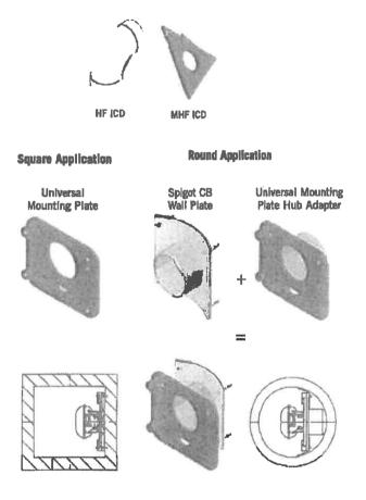
The HF Sump is available to accommodate low to no sump applications in both square and round catch basins:
