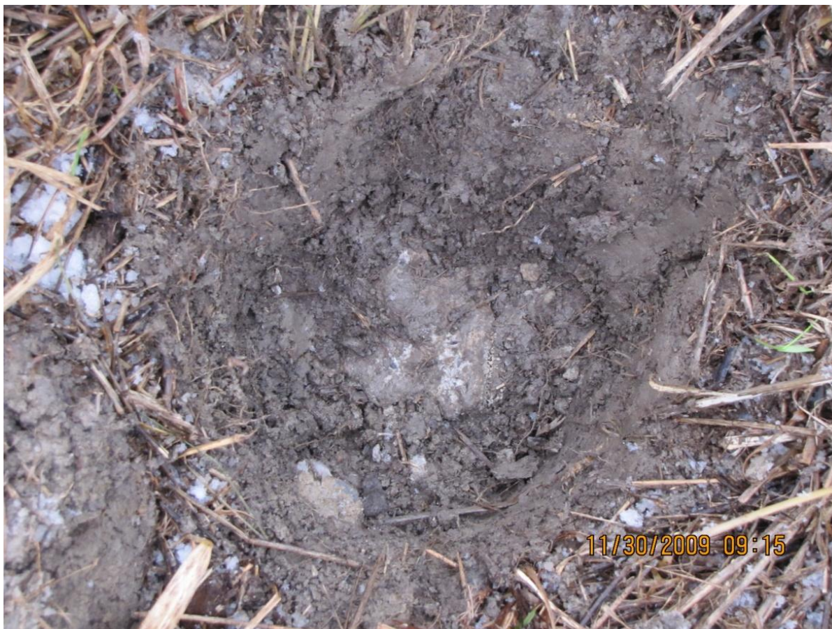
Plate 17: Test pit in section 6G showing grey clay soil and concrete at the bottom of the test pit.
