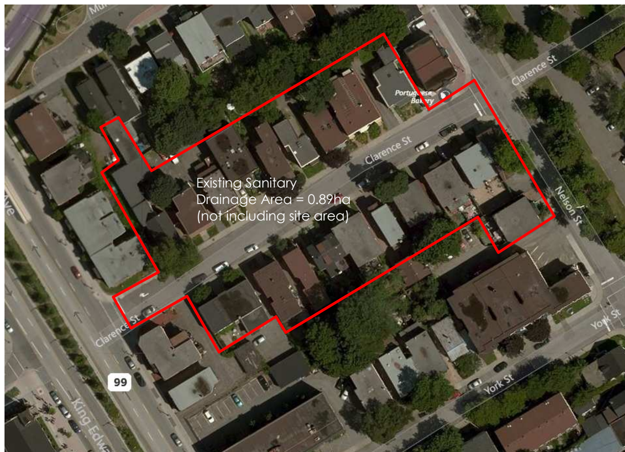
Figure 2: Existing Sanitary Drainage Area
