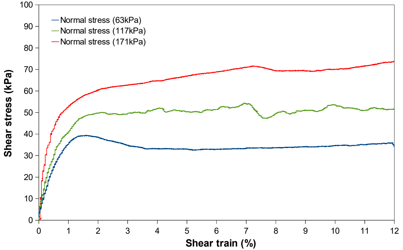
Figure 7: Stress-strain curves obtained from consolidated drained direct shear test
