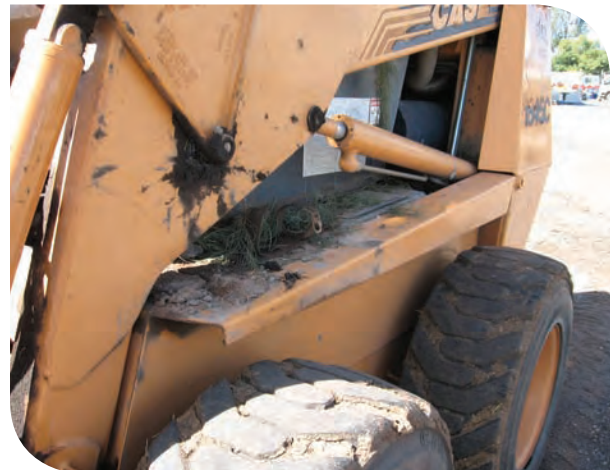
Plant material attached to bobcat.
