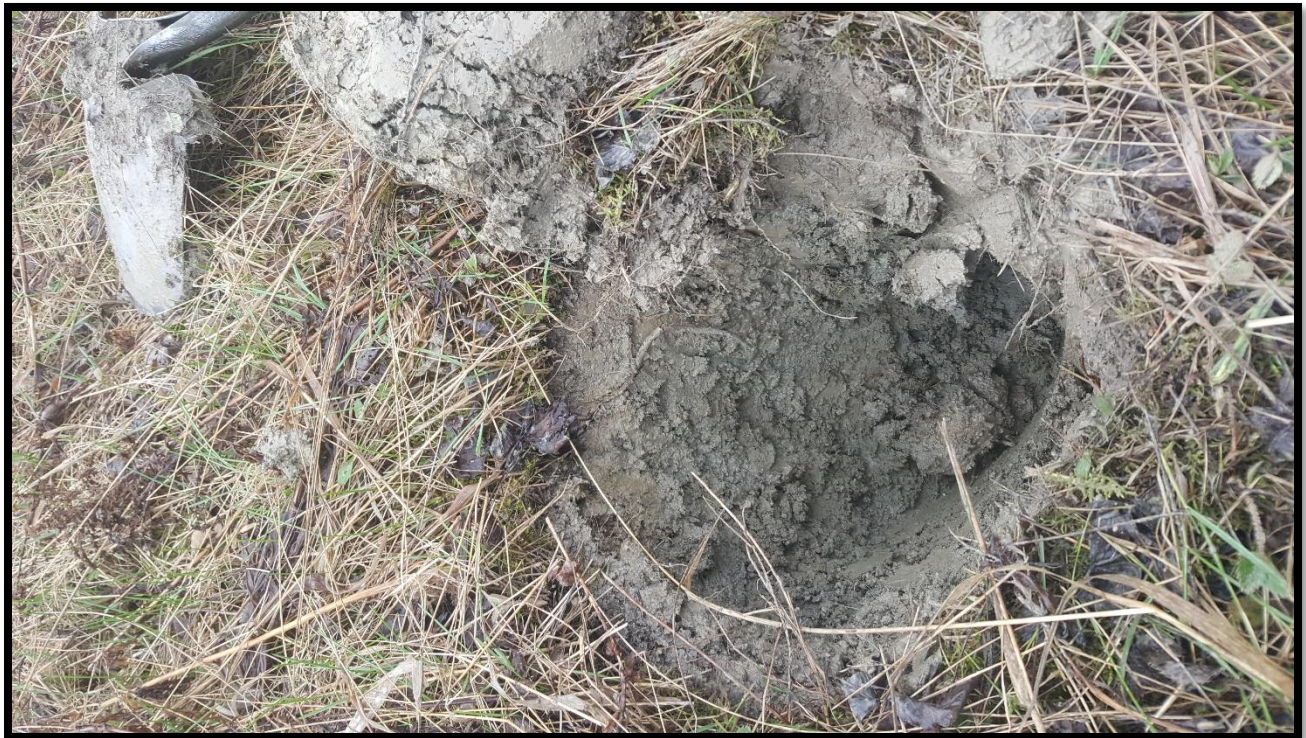
Figure 4: Typical test pit in progress (D04).
